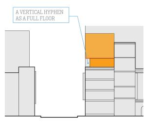
Indent or setback new floors that sit above retained elements to highlight the change in structure, space, and age of new construction.
