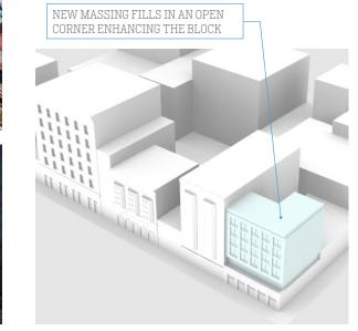
Use the additional massing to help a smaller building join the scale and patterns of the block.
