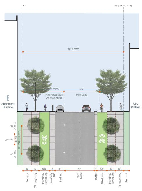
Figure 5.13-6: Lee Avenue, Section 2 \*see "Figure 5.13-4 & 5: Lee Avenue, Plan Enlargements L.2 & L.3
