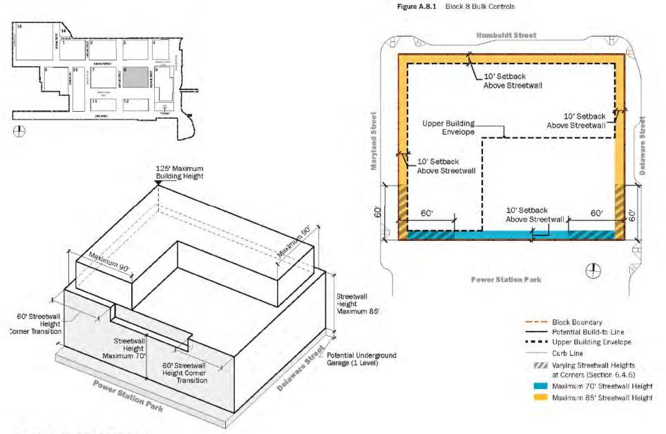
Figure A.8.2 Block 8 Bulk Controls Axon
