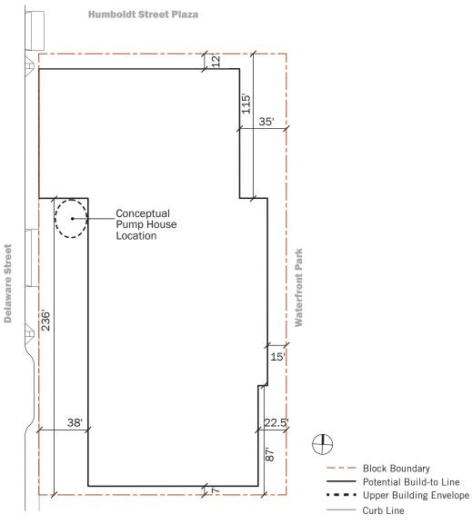
Note: Above a height of 36 feet, the building may project west of the 38-foot setback line by up to 17 feet, provided that SFFD can adequately service the building.
