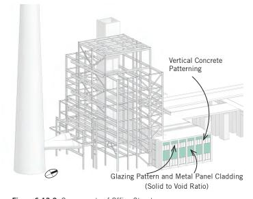
Figure 6.13.2 Components of Office Structure
