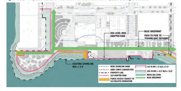
Figure 4.3.3 Typical Existing and Proposed Shorelines at Riprap and Seawall
