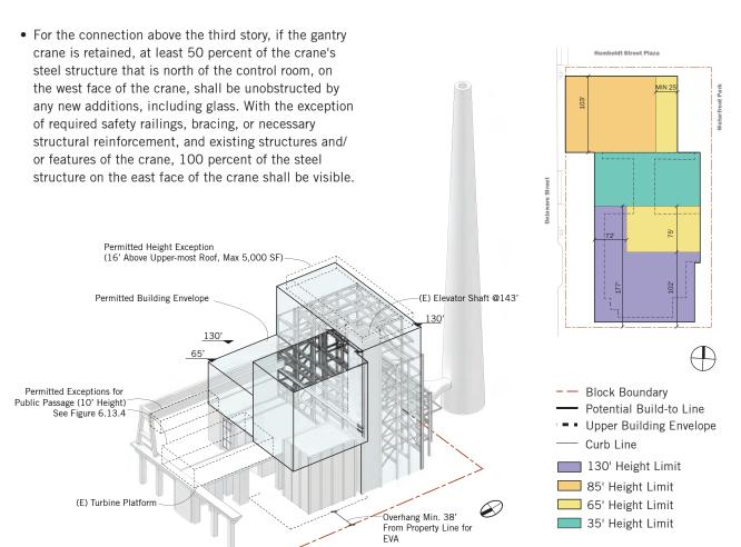
Figure 6.13.3 Unit 3 Massing and Block 9 Height Diagram
