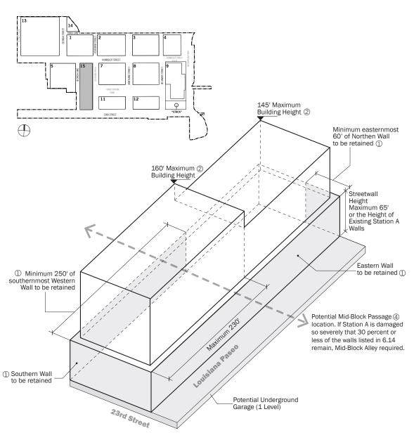
Figure A.6.2 Block 15 Bulk Controls Axon
