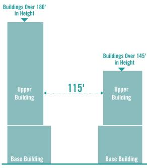
**Figure 6.5.6** Upper Building Separation for Midrise and Highrise Towers on Different Blocks
