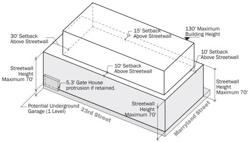
Figure A.10.2 Block 11 Bulk Controls Axon
