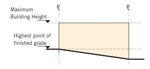
Figure 6.2.2 Measuring Height on a Slope
