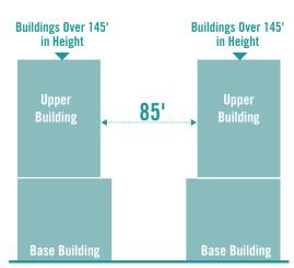
Figure 6.5.5 Upper Building Separation for Midrise Towers on Different Blocks
