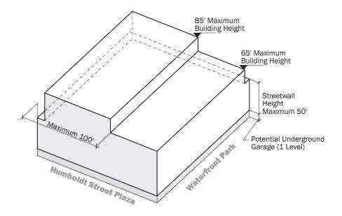
Figure A.4.2 Block 4 Bulk Controls Axon
