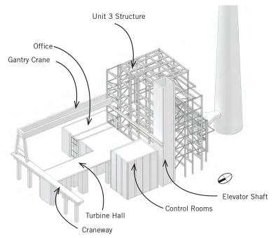
Figure 6.13.1 Components of Unit 3
