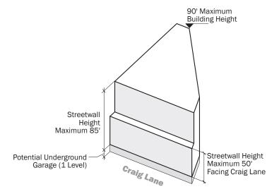
Figure A.13.2 Block 14 Bulk Controls Axon
