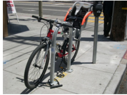
Acceptable These bicycle racks provide two points of support for bicycles. They are constructed with square tubed material which makes the racks resistant to cutting.
