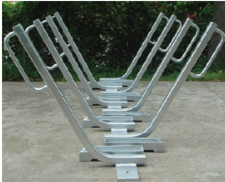
Acceptable These bicycle racks provide two points of support for bicycles. They are constructed with square tubed material which makes the racks resistant to cutting.
